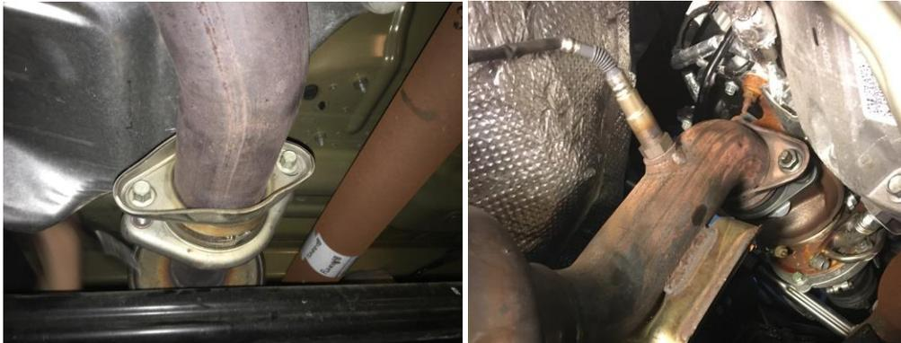
Step 3: Remove the two bolts that connect the downpipe to the resonator pipe.
