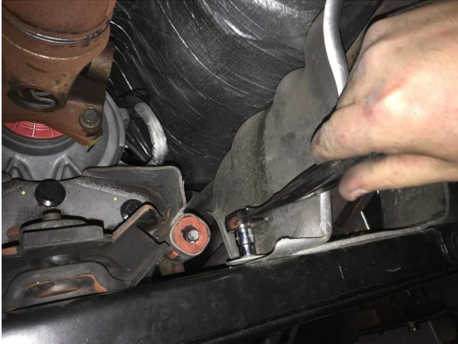
Step 2: Things will be a lot easier if you remove the shield that attaches to the transmission cross member and goes up and over the downpipe.
